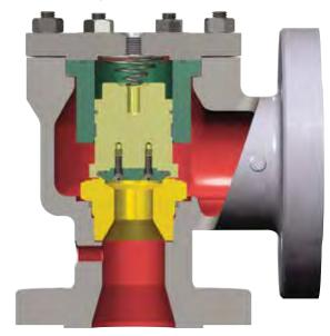
Because of its modular design, the 39PV (pop action pilot) can be converted to a 39MV (modulating action pilot), making GE's Consolidated 39PV/39MV pilot valve one of the most versatile pilot valves available today.
