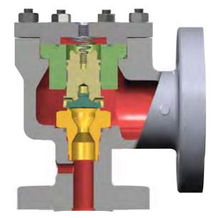
The Consolidated 3900 series pilot-operated safety relief valve from GE is supplied with a non-flowing pilot valve. This single pilot design is well-suited for both incompressible and compressible applications and performs equally well on liquid, vapor or two-phase flow services. The set pressure will not require adjustment if service conditions change.
